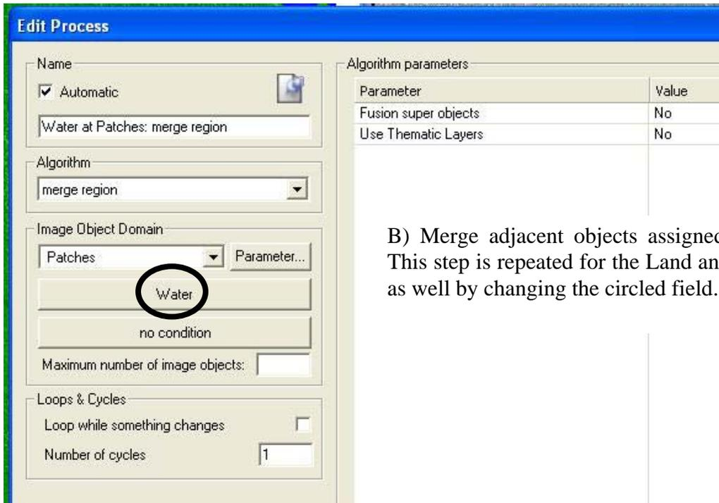
B) Merge adjacent objects assigned the class of Water. This step is repeated for the Land and Wetter Area classes as well by changing the circled field.
