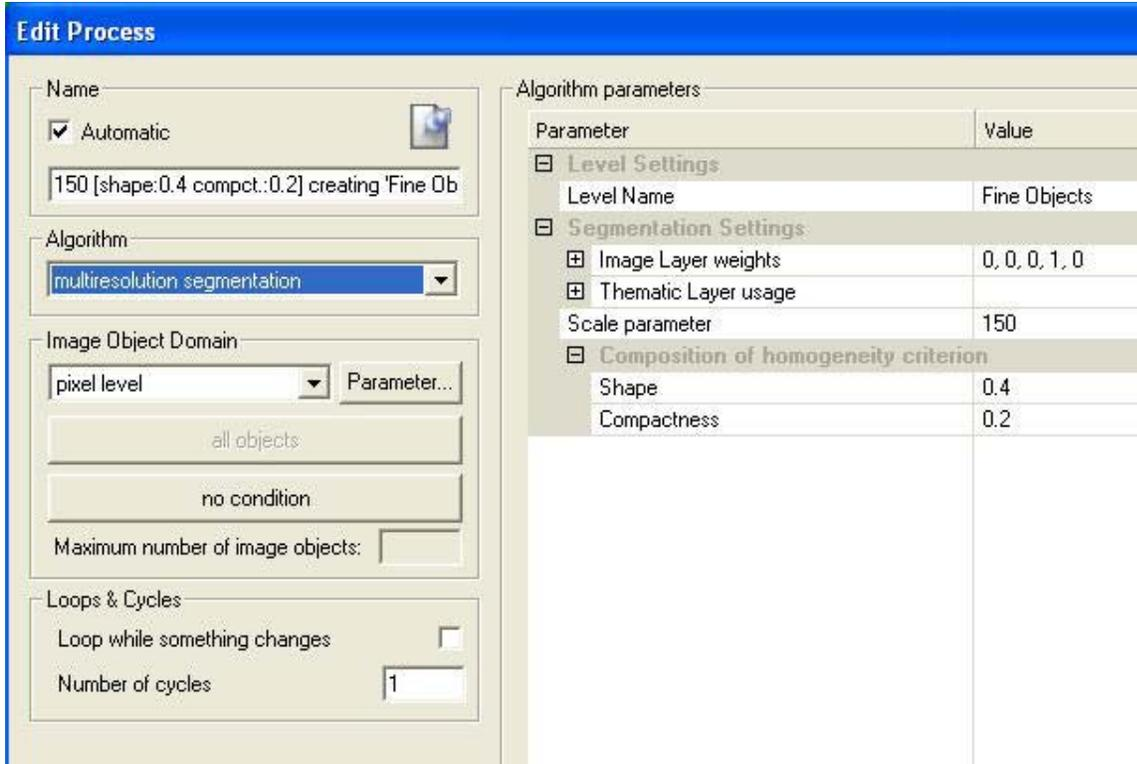
Fig. 2a: Multiresolution segmentation parameters for coastal area.
